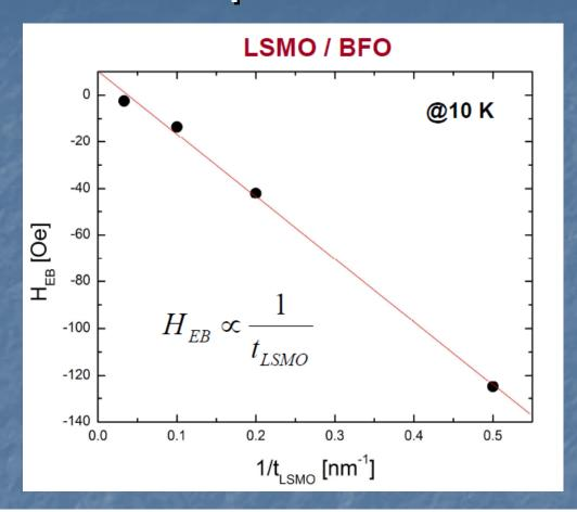
Exchange Bias interaction between La<sub>0.7</sub>Sr<sub>0.3</sub>MnO<sub>3</sub> and BiFeO<sub>3</sub>
