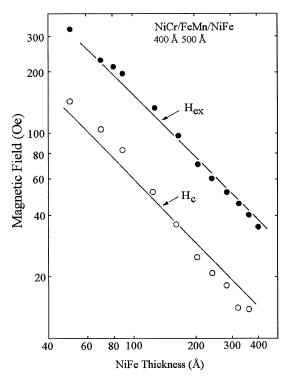
Fig. 9. Dependence of exchange bias  $H_{\rm E}$  (filled symbols) and coercivity  $H_{\rm C}$  (open symbols) with the FM layer thickness for Fe<sub>80</sub>Ni<sub>20</sub>/FeMn at a fixed  $t_{\rm AFM} = 50$  nm [208].
