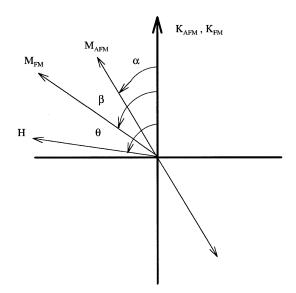
Fig. 8. Schematic diagram of angles involved in an exchange bias system. Note that the AFM and FM anisotropy axes are assumed collinear and that the AFM sublattice magnetization  $M_{\rm AFM}$  has two opposite directions.
