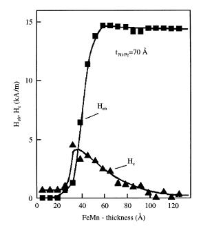
Fig. 10. Dependence of exchange bias  $H_{\rm E}$  (square symbols) and coercivity  $H_{\rm C}$  (triangular symbols) with the AFM layer thickness for Fe<sub>80</sub>Ni<sub>20</sub>/FeMn at a fixed  $t_{\rm FM} = 7$  nm [15]. Note that 80 A/m = 1 Oe.
