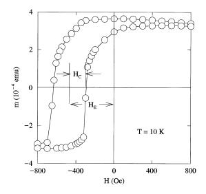
Fig. 1. Hysteresis loop, m(H), of a FeF<sub>2</sub>/Fe bilayer at T = 10 K after field cooling [72]. The exchange bias,  $H_{\rm E}$ , and the coercivity,  $H_{\rm C}$ , are indicated in the figure.
