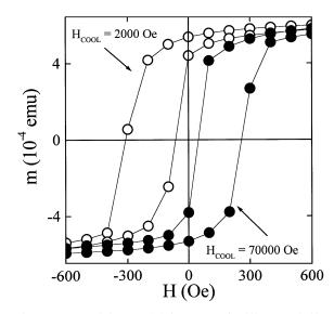
Fig. 14. Hysteresis loops, m(H), for an FeF<sub>2</sub>/Fe bilayer cooled in  $H_{\text{COOL}} = 2000 \text{ Oe}$  (open symbols) and  $H_{\text{COOL}} = 70\ 000 \text{ Oe}$  (filled symbols), at T = 10 K [91].
