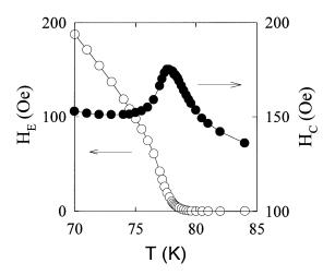
Fig. 13. Exchange bias,  $H_{\rm E}$ , and coercivity,  $H_{\rm C}$ , versus temperature for an FeF<sub>2</sub>/Fe bilayer after field cooling.
