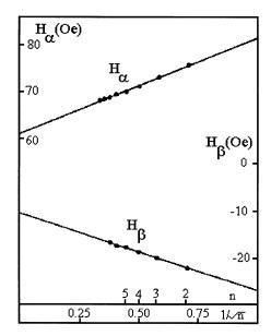
Fig. 12. Coercive fields for the increasing field branch,  $H_{a}$ , and decreasing field branch,  $H_{\beta}$ , of the hysteresis loop as a function of measurement order, *n*, for an Fe<sub>20</sub>Ni<sub>80</sub>/FeNiMn bilayer at room temperature [218].
