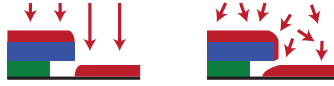
Figure 4.3: Schematics of two different types of metal deposition: metal evaporation and ion sputter deposition. The substrate is covered with a bilayer resist (the green and blue bars).
