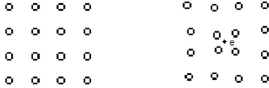
Figure 2.1: The lattice distortion caused by a passing electron.
