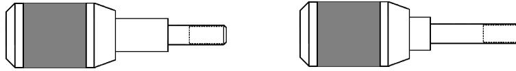
Figure 223-1 Stabilizing screw for securing the vertical scanner to the support ring. MultiMode AFM screw (left), and screw for other SPMs (right).
